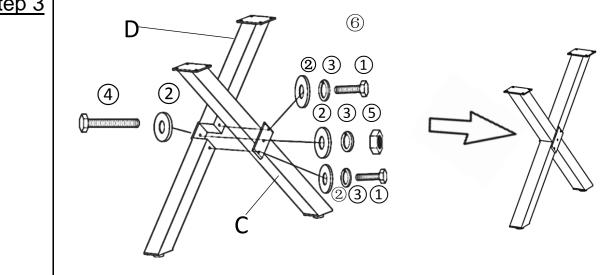
Repeat the same assembly process for the other Inner Table Legwith Pre-attached Leveller(C) and Outer Table Leg with Pre-attachedLeveller(D).
