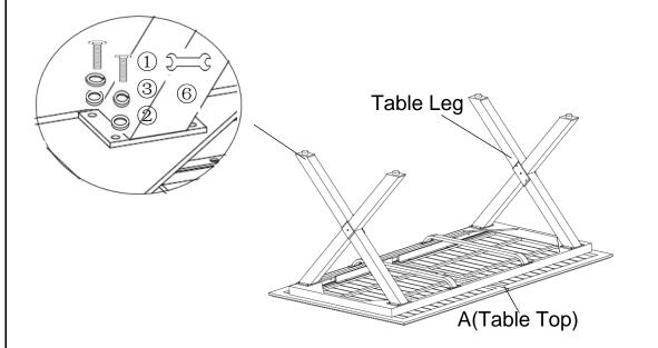
Turn the table upside down on to a soft surface that does not scratch the tabletop.
