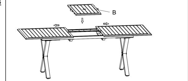
To expand the Table, pull the table top apart, place Table Top Extension Leaf (B) into the middle leaf slot. Adjust the direction/angle to tightly fit into the housing in the Table Top.
