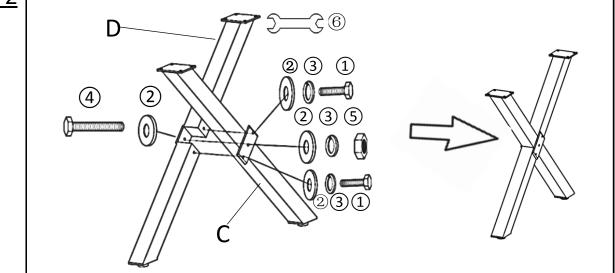
Fix the Inner Table Leg with Pre-attached Leveller(C) and Outer Table Leg with Pre-attached Leveller(D) with bolts(4), washers(2), spring washers(3) and nuts(5) by spanner(6).
