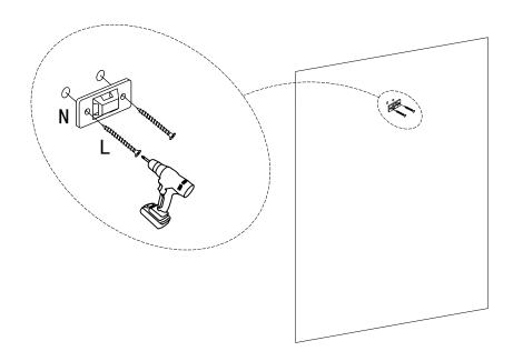
Move the Bookcase back against the wall. Fix Metal Bracket (N) on the bottom of Long Shelf (E) using Short Screw (M) with Drill Bit (not provided). Pull the Restraint Strap (O) through the Metal Bracket (N) on the wall and Long Shelf (E) and pull the Restraint Strap (O) tight.
