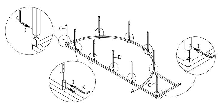
Attach Front Frame (B) to Top and Bottom Rail (C) and Rail (D) using Bolt (I) with Allen Key (K).
