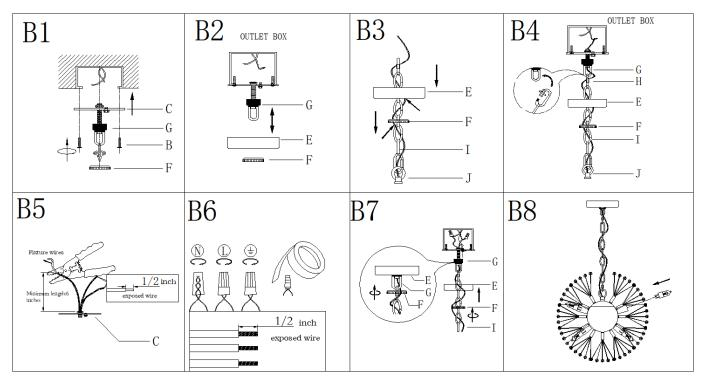
Step B1: Remove the collar ring (F) from collar loop (G). Attach the single bar (C) to the outlet box with mounting screws (B). **Note:** the side of single bar marked "GND" must face out.
