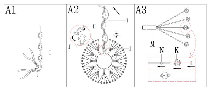
Step A1: By measuring, determine the correct number of links needed for proper hanging height. Using the chain pliers, disconnect and discard the unwanted part.
