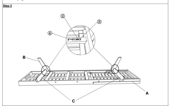
With the assistance from your adult partner, attach the Cross Bar (C) to the Seat Panel (A) and the Leg Panel (B) of the assembled part in Step 2 by using Bolt ((2)), Washer ((3)) and Allen Wrench ((4)) as shown above. **Do not fully tighten the Bolts.**
