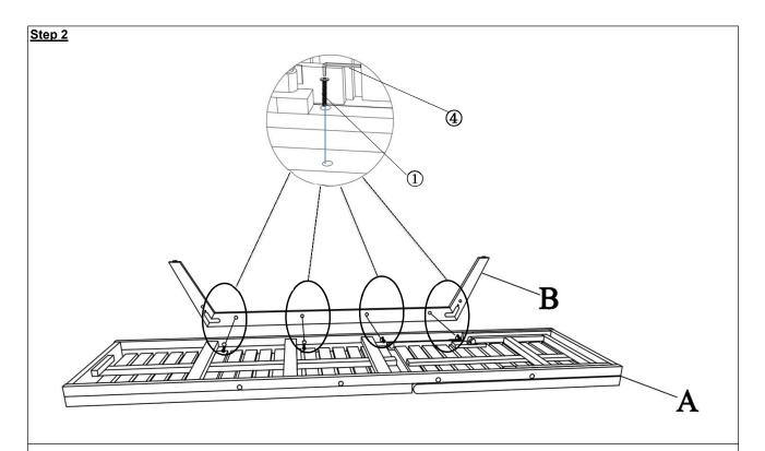
With assistance from your adult partner, place the Seat Panel (A) facing up on a clean, non-marring surface. Attach the Leg Panel (B) to the Seat Panel (A) by using Bolt (1) and Allen Wrench (4) as shown above. **Do not fully tighten the Bolts.**
