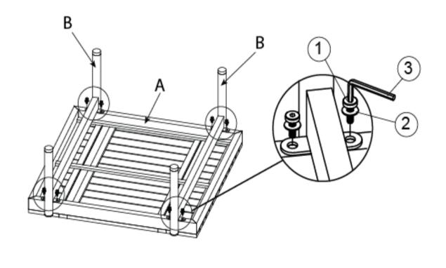
Place the Table Top(A) facedown onto a clean, non-marring surface as shown in picture above.
