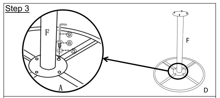
Attach the Support Ring(F) to the Table Top (D) using Bolts(®) and Washers(⑤) with the Allen Key(⑨).
