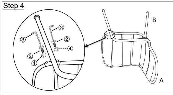
Align the mounting positions on the Chair Leg(B) and Chair Seat(A), then attach using Bolts(2) and Washers(4)with the Allen Key(3).
