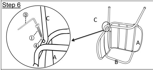
Align the mounting positions on the Chair Leg(C) and Chair Seat(A), then attach using Bolts(1) and Washers(4)with the Allen Key(3).(Here are two positions that need to be assembled)
