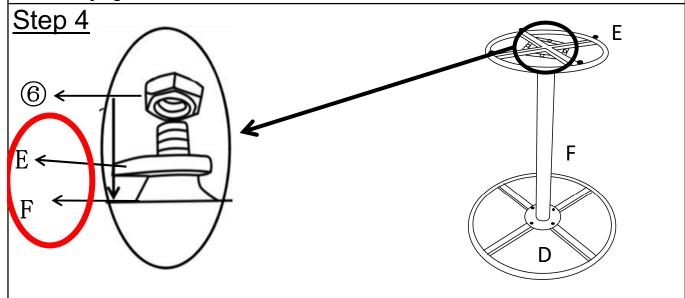
Attach the Support Ring(F) to the Table Base(E) using Nuts(6) with the Spanner wrench(7). **Tighten all Nuts at all joints in a sequential manner.**
