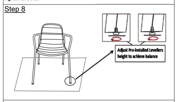
Adjust the Pre-installed Levellers at the base of the Legs until the Chair is level with the ground.
