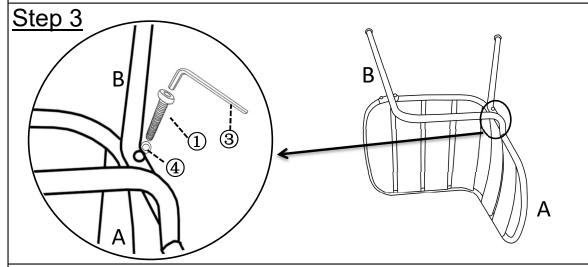
Align the mounting positions on the Chair Leg(B) and Chair Seat(A), then attach using Bolts(①) and Washers(④) with the Allen Key(③). (Here are two positions that need to be assembled)
