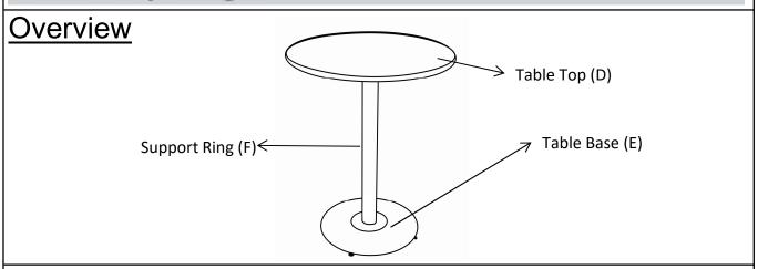
This Table has multiple parts and may require up to 20 minutes to assemble. To give you an overview of the Table parts, the above picture is to help you put the various parts into perspective. Please read through the instructions below to familiarise yourself with the parts and steps before assembly.
