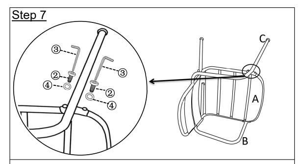
Align the mounting positions on the Chair Leg(B) and Chair Seat(A), then attach using Bolts(2) and Washers(4)with the Allen Key(3). **Tighten all Bolts**.
