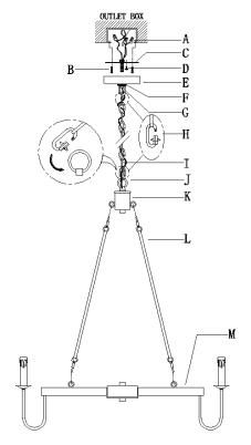
Step A1: Adjust the arms (M) to the proper position.
