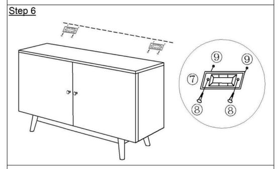
Attach Brackets (⑦) to Wall Plugs (⑨) using Wall Plug Screws (⑧) with Screwdriver (④).
