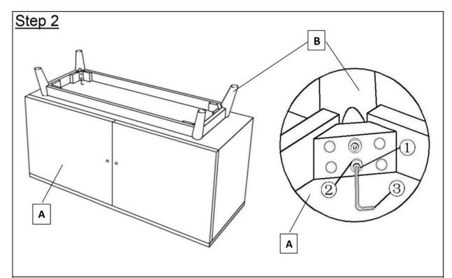
As shown in "Step 2" picture Affix the Leg (B) in to the Top (A) by using Allen Bolt (1), Washer (2) and Allen Key (3).
