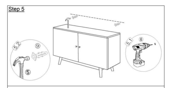
5.1) Drill two holes on wall at same height as Brackets (7) on Cabinet with Power Drill (6).
