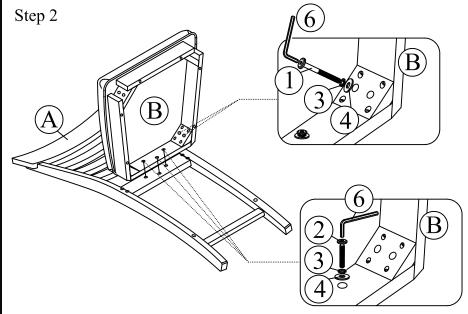
Step 1: Place Chair Back (A) on the floor. Attach Seat Box w/Seat Cushion (B) to Chair Back (A) by using the Flat Washer (4), Lock Washer (3), Long Bolt (1) into the holes at the rear corner block of the seat box and secure by Allen Key (6). Insert Flat Washer (4), Lock Washer (3), Short Bolt (2) into the holes at the rear bar of the seat frame. Tighter all Bolts with Allen Key (6). Do not fully tighten.
