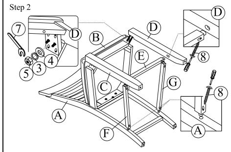
Step 2: Attach the LSF/RSF Front Leg (C/D) to Seat Box w/Seat Cushion (B) by using Lock Washer (4), Lock Washer (3) and Hex Nut (5) secure by Open Wrench (7). Attach the Front/LSF/RSF Side Stretcher (E/F/G) to LSF/RSF Front Leg (C/D) and Chair Back (A) by securing the Screw (8) with Phillips - head screw drivers (Not provided).
