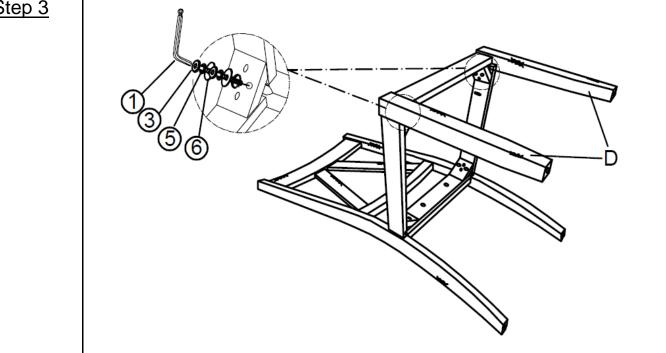
Attach Front Leg (D) to Seat Frame (C) using Bolt (3), Spring Washer (5) and Washer(6) with Allen Wrench (1). Do not fully tighten the Bolts.
