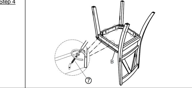
Then, turn the Dining Chair upside down and fix the Cushion Seat (B) using Screw (7) with Screwdriver (Not Provided).
