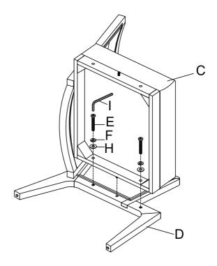
3 Attach Seat (C) to Left Arm Frame (B), using Bolt (E), Lock Washer (F) & Flat Washer (H) by Allen Key (I) as below shown.
