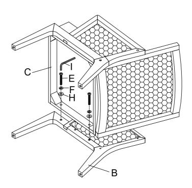
Assemble Left Arm Frame (B) with Back Frame (A), using Bolt (E), Lock Washer (F) & Flat Washer (G) by Allen Key (I) as below shown.
