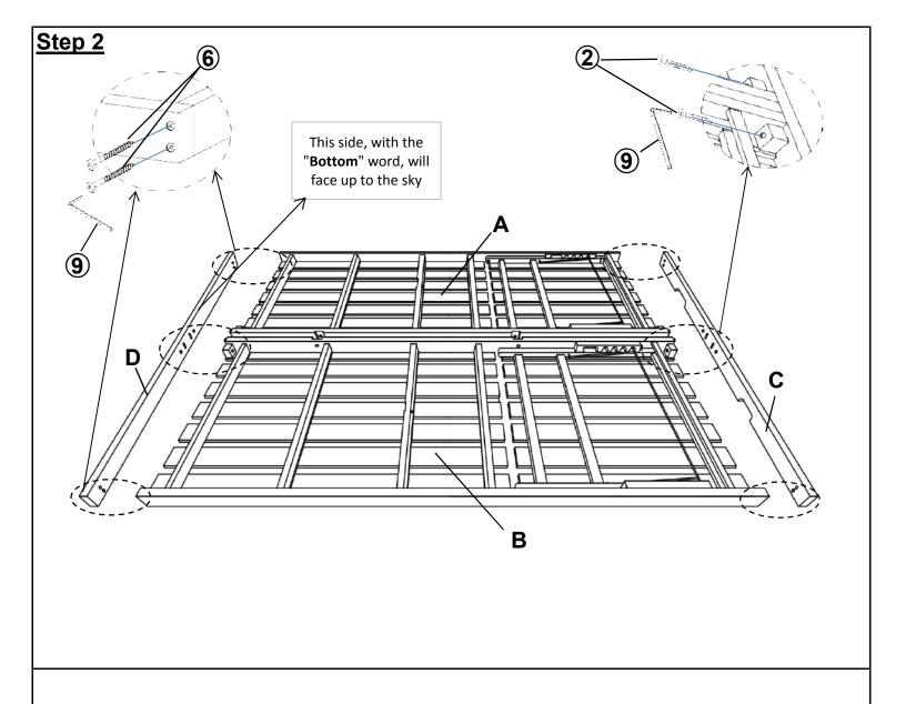
Place the Right Foldable Seat Panel (A), and the Left Foldable Seat Panel (B) face down onto a clean, non-marring surface.
