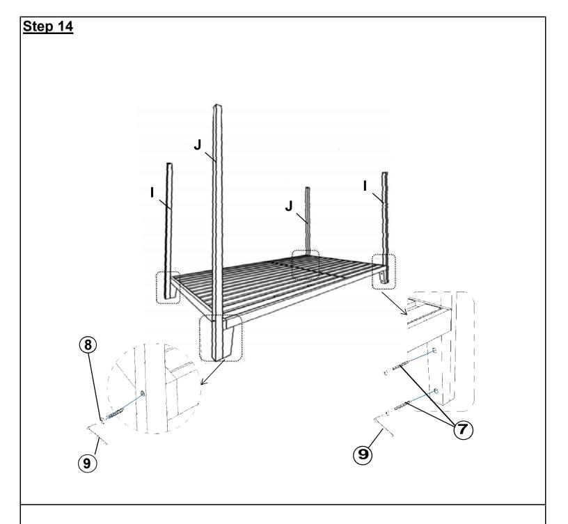
With assistance from your adult partners, take the Second Leg Bars (I) and the First Leg Bars (J) out of the assembled part in Step 13 by using the Allen Wrench (9) to remove the Screws (8) and Screws (7) as shown above
