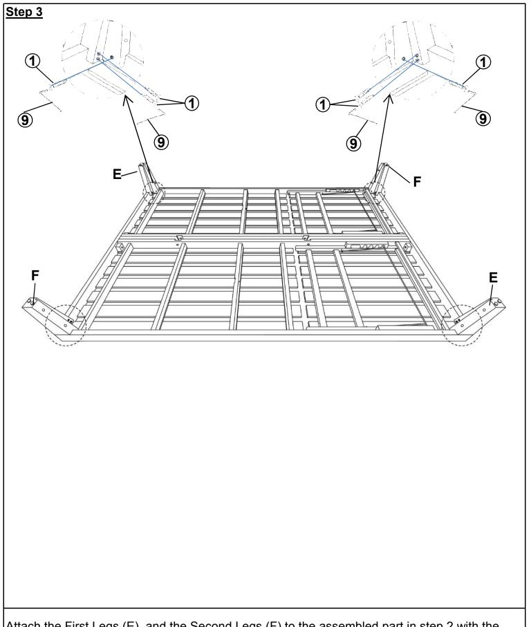
Attach the First Legs (E), and the Second Legs (F) to the assembled part in step 2 with the Bolts (1) and the Allen Wrench (9) as shown above.
