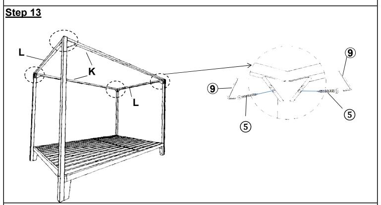
By taking a Step Ladder or an A-frame Ladder as well as with assistance from your adult partner, take the Long Top Bar (K) and the Short Top Bar (L) off of the assembled part in step 12 by using the Allen Wrench ((9)) to remove the Screws ((5)) as shown above
