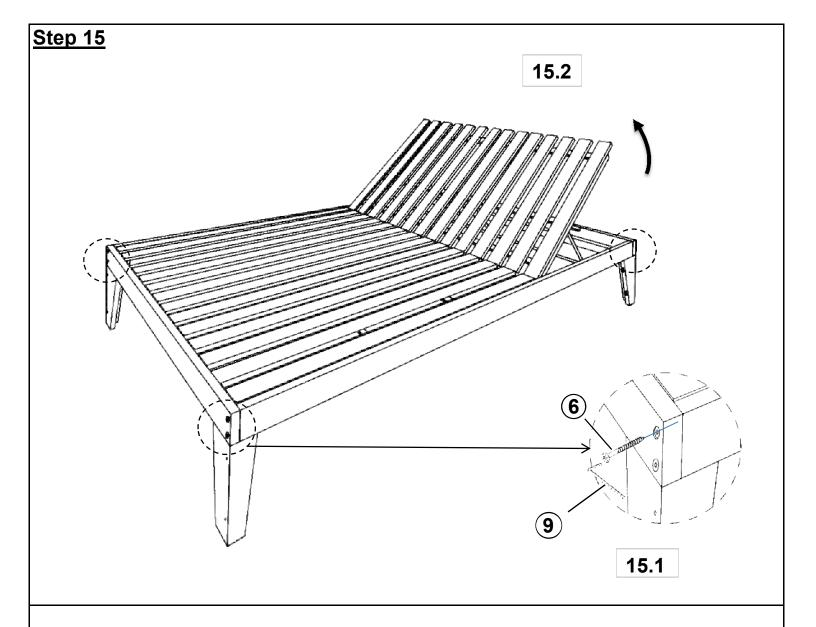
**15.1.** Insert the Screws (6) into the upper holes at the 4 corners of the Upper Seat Bar (C) and the Lower Seat Bar (D) in the assembled part in Step 14 by using the Allen Wrench (9) as shown above.
