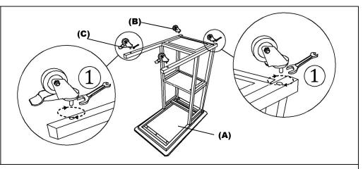
Keep the TABLE(A) inverted on the clean surface and bottom facing the top then place the WHEEL(WITHOUT LOCK)(B) on designated points at back side of TABLE(A) as shown above and tighthen it by using Spanner((1)). Repeat the same process with other WHEEL L(WITHOUT LOCK)(B) AND WHEEL WITH LOCK (C).
