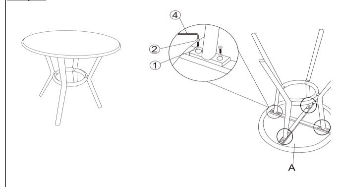
Attach one of the Legs(B) to the Table top (A) with the Bolts(2) and washers (1 Key(4) as shown above.
