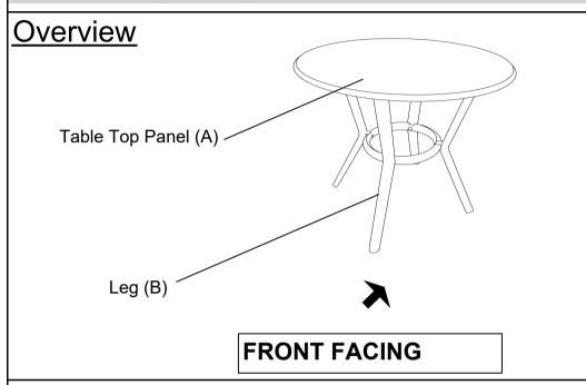
This Table has multiple parts and may require up to 30 minutes to assemble. I overview of the Table parts, the above picture is to help you put the various pa Please read through the instructions below to familiarise yourself with the parts assembly.
