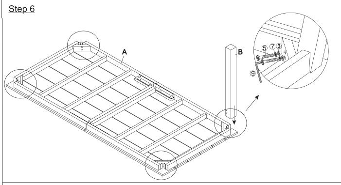
Attach the Legs (B) into the mounting position at the corners of the Table Top (A), using the Bolts (5) with Spring Washers (7), Washers (3) and Allen Key (9) as shown in the picture.
