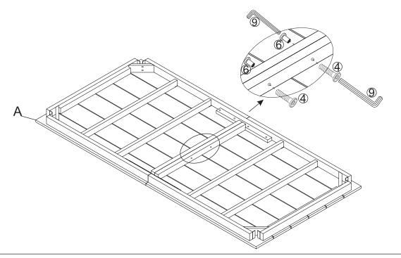
Secure Table Top (A) using the Bolts (4), Sleeve Nut (6) and Allen Key (9) as shown in the picture.
