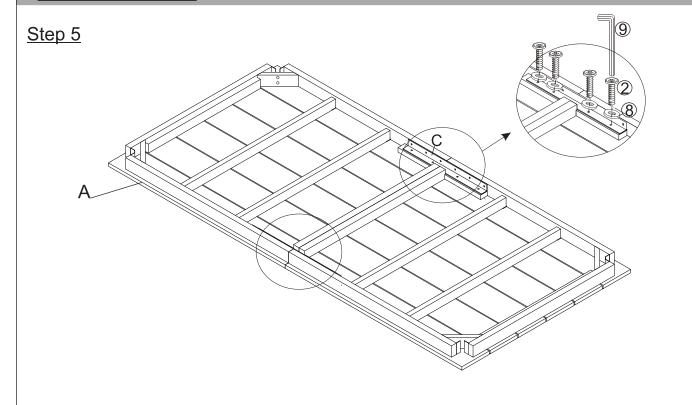
Secure Support Bar (C) to Table Top (A) using the Screws (2), Washer (8) and Allen Key (9) as shown in the picture.
