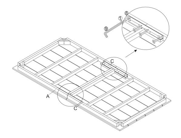
Place Support Bar (C) to the housings of Table Top (A) secure by using the Bolts (1) with Washer (8), and Allen Key (9) as show in picture above.
