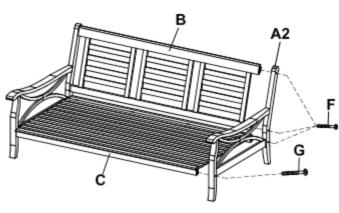
Attach back support (B) and seat (C) into right side frame (A1). Secure using 1 1/2" Bolt (F) on back leg and 2" Bolt (G) on front leg. Tighten all bolts using screwdriver.
