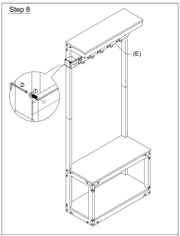
Take the Hanger Strip (E) and align it with matching holes of Top (D). Tighten the Flat Head Allen Bolt (1) with the help of Allen key (2) as shown in the picture above.
