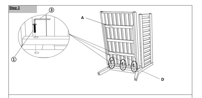
Attach the Seat Panel (A) to the Left Leg Panel (D) of the assembled part in step 2 by using Bolt (1) and Allen Wrench (3)
