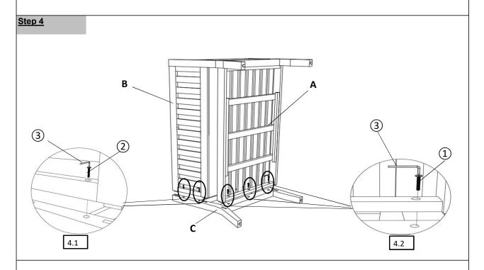
With assistance from your adult partners, flip up the assembled part in Step 3 to attach to the Right Leg Panel (C) 4.1. Attach the Right Leg Panel (C) to the Backrest Panel (B) of the assembled part in step 3 by using Bolt (2) and Allen Wrench (3)
