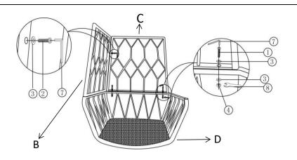
Assemble Middle Back (C) and Seat (E) by using Bolt (①), Nut (④) Washer (③) with Allen Key (⑦) and Wrench (⑧). Then assemble Middle (C) and Left Back (B) by using Bolt (②) and Washer (③) with Allen Key (⑦). Do not tighten.
