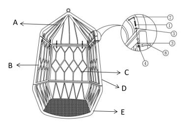
Assemble Top (A) and three back panels (B, C, D) by using Bolt ( 1 ), Nut (4) Washer ( 3 ) with Allen Key ( 7 ) and Wrench ( 8 ). Do not tighten.
