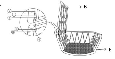
Unpack and place all parts on a clean surface. Assemble Left Back (B) and Seat (E) by using Bolt (1), Nut (4) Washer (3) with Allen Key (7) and Wrench (8). Do not tighten.
