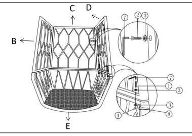
Assemble Right Back (D) and Seat (E) by using Bolt (1), Nut (4) and Washer (3) with Allen Key (7) and Wrench (8). Then assemble Right Back (D) and Middle (C) by using Bolt (2) and Washer (3) with Allen Key (7). Do not tighten.
