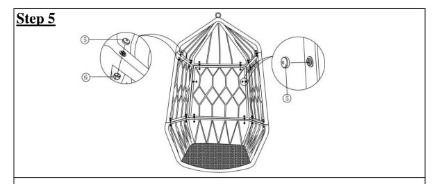
Tighten all screws and nuts . Then add the Nut Caps ( (5), (6)) on all the Bolts .
