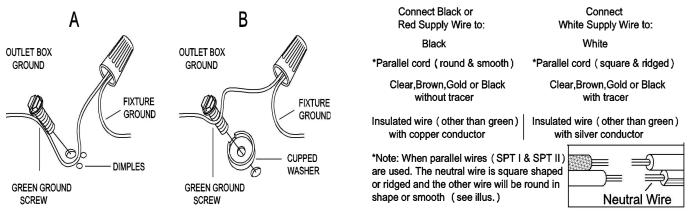
Twist plastic wire connector until wires are tightly joined together, wrap each connector with approved electrical tape. Be sure that no wire strands are exposed and then carefully tuck all wires into the outlet box.
