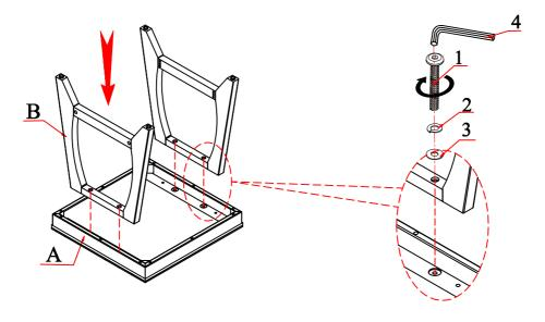
Step 2: Attach the Stretcher (C) to the Leg (B) by using Flat Washer (3), Lock Washer (2) and Bolt (1). Secure well by Allen Key (4), fully tighten bolts at this time then attach the wood plug (5). Product assembly is now complete.
