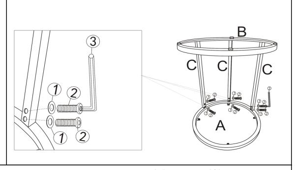
Align the mounting positions on the Table Top(A) and Leg(C), then attach using Washers(1) and Bolts(2) with Allen Key(3) as shown. Do not fully tighten the Bolts.
