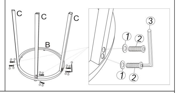
Align the mounting positions on the Support Bar(B) and the Leg(C), then attach using Washers(1) and Bolts(2) with Allen Key(3) as shown. **Do not fully tighten the Bolts.**
