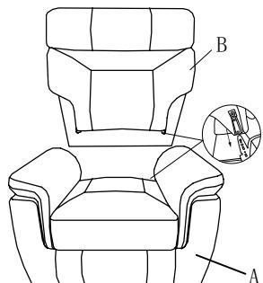
Step 3. Please insert the LSF ear and RSF ear to the back rest and make sure it is secured in position.
