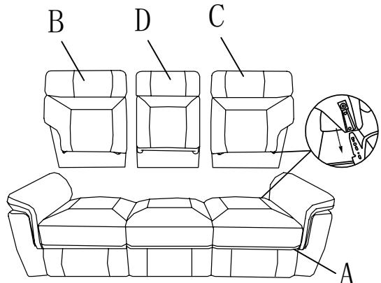
Step 2. Please insert the LSF ear and RSF ear to the back rest and make sure it is secured in position.
