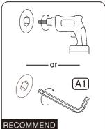
Recommend using a power tool to only tighten hardware (#1) faster.
