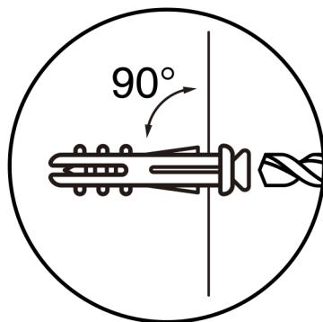
4. Take extra care when drilling into high walls or ceramic tiles. Wall anchors should be a tight fit for the hole. Never use wall anchors in ceilings.
