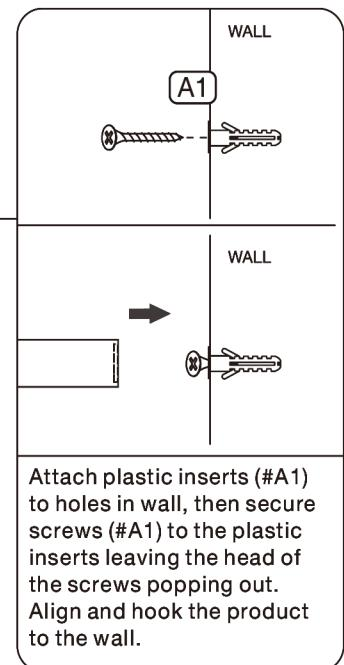
Attach plastic inserts (#A1) to holes in wall, then secure screws (#A1) to the plastic inserts leaving the head of the screws popping out. Align and hook the product to the wall.
