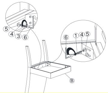
Attach front legs (C) to the seat frame. Use bolks (2), washers (4) and (5). Tighten with Allen Key (6). Attach bottom removed on the step 1 on seat frame.
