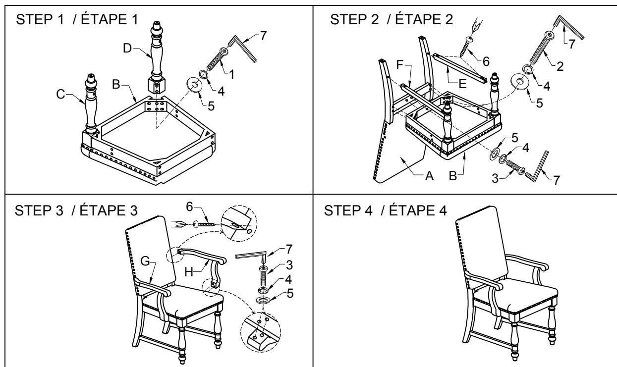
DONOT TIGHTEN BOLTS UNTIL COMPLETELY ASSEMBLED.
