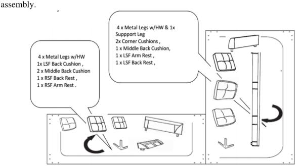
**Step 1** Align the legs to the pre-drilled holes at the bottom of the units, insert bolts and washers then tighten with Allen Key. Rotate support leg Q to tighten it.
