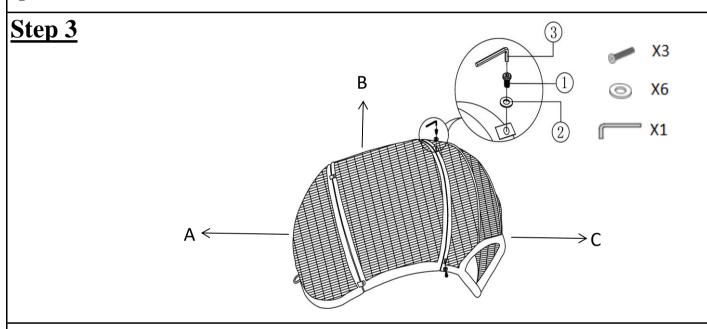
Proceed to assemble Seat (C ) and Back (B) by using Bolt ( ① )and Washer ( ② )with Allen Key ( ③ ) . Do not tighten.
