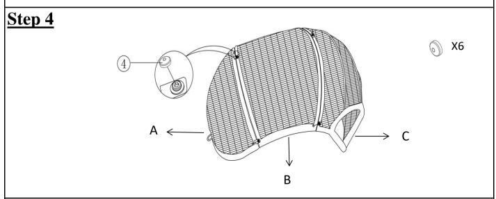
Tighten all screws and nuts . Then add the Nut Caps( 4 ) on the 6 Bolts as shown in the picture above.
