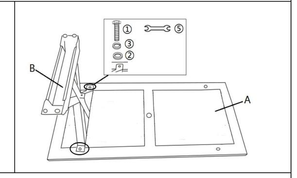
Lay the Table Top(A), facedown onto a flat, clean, non-marring surface. Attach Table Leg with pre-attached Leveller(B) to Table Top(A) using Washers(②), Spring Washers(③), and Hex Bolts(①) with Spanner(⑤). **Do not fully tighten the Bolts.**
