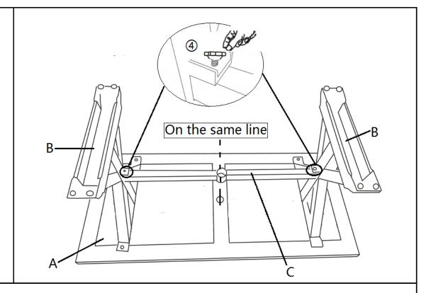
Align the mounting position on Table Leg with pre-attached Leveller(B) to Supporting Rod(C).
