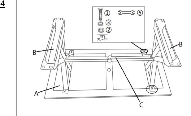
Insert the Support Rod(C) into the other Table Leg with pre-attached Leveller(B). Then attach the Table Leg with pre-attached Leveller(B) to Table Top(A) using Washers(②), Spring Washers(③), and Hex Bolts(①) with Spanner(⑤).
