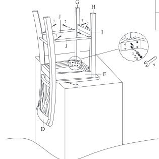
Attach chair left and right front legs (G & H) to seat frame (F) with flat washers (3), spring washers (2), and nuts (8) as shown. Do not fully tighten nuts (8). Insert chair left side crossbar and chair right side crossbar (J) into the front left and right chair legs (G & H) and chair back frame (D).
