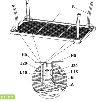
Connect the table top (A) and the legs (B) with 8 bolts (J20), 8 washers (L15). Do not over-tighten them.
