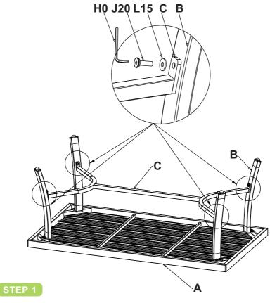
Attach the support bar (C) to the legs, using 4 bolts (J20) and 4 washers (L15). Do not over-tighten them.
