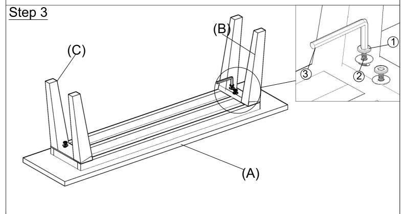
Repeat the above process with second Right Leg (B) and fully tighthen the bolts.
