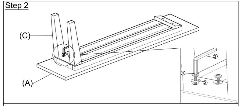
Place the Top (A) with top side face skywards onto a clean, soft surface to avoid any scratches or damages to the product. Align the Left Leg(C) with connector screw hole in Top(A) as shown above.
