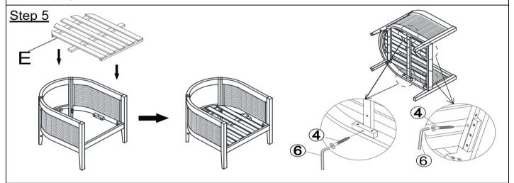
With assistance from your adult partner(s), attach the **Seat Panel (E)** into the assembled frame in step 4. Achieve this by using **Screws (4)** and the **Allen Wrench (6)**, as shown in the above picture.
