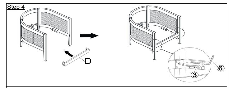
With assistance from your adult partner(s), attach the **Front Apron Support Bar (D)** to the assembled frame in step 3. Achieve this by using **Bolts (3)** and the **Allen Wrench (6)**, as shown above.
