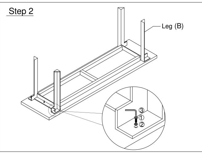
Take the Leg (B) and align it with the holes on the bottom, then insert the Flat Head Allen Bolt (1) along with the Washers (2) and tighten it with the help of Allen key (3) as shown in the picture above. Repeat the same step and attach the other Leg.
