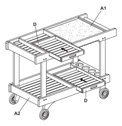
Attach the trays (D) to the section Top frame (A1) and bottom frame (A2).
