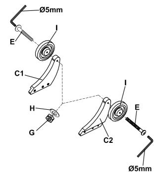
Attach wheel (I) on to right & left bottom leg (C1&C2). Insert 3" Bolts (E), Spring washer(H), and nut (G) hold on the bolts using  $\varnothing 5 \text{mm}$  Allen wrench, and tighten nut using wrench.
