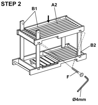
Attach long legs (B1) and short legs (B2) onto top frame (A1). Insert 1 1/2" Bolts (F) using Ø4mm Allen wrench. As picture shown.
