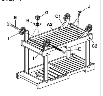
Attach right and left bottom leg (C1&C2) which has wheels attached on to Bottom frame (A2) secure using 1" screws (J).
