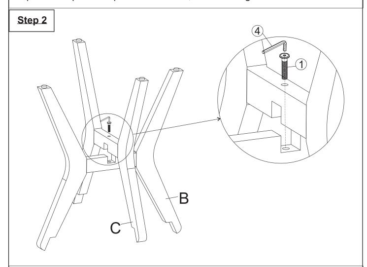
Position the First Leg Frame (B) to the Second Leg Frame (C) as shown in the above picture. Secure the First Leg Frame (B) to the Second Leg Frame (C) by using a Bolt (1) and the Allen Key (4).
