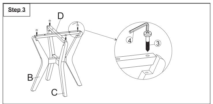
Turn the assemble in step 2 right side up Attach Support Panel (D) to First Leg Frame (B) and Second Leg Frame (C) from Step 2, using a Screw (③) and Allen Key (④). **Do not fully tighten the Bolts.**
