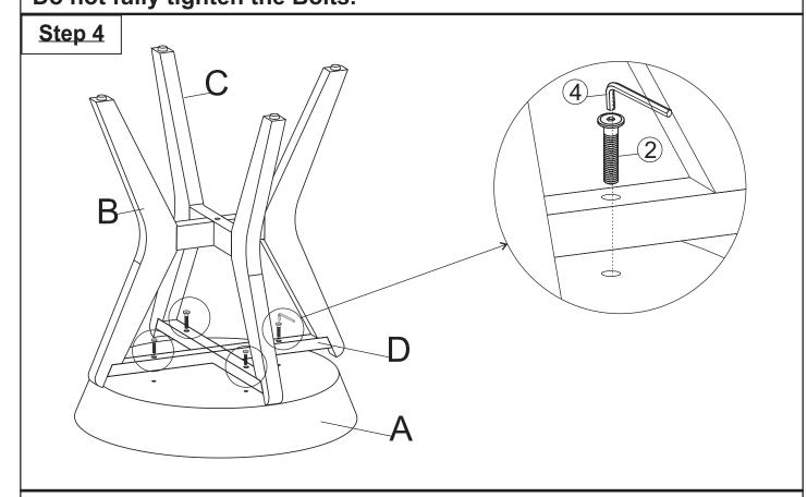
Place the Table top (A) with its underside skywards onto a clean, soft surface to avoid any scratches or possible damage to the product. Position the assemble from step 3 onto the Table Top (A), by using a Bolt (2) and the Allen Key (4).
