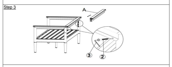
Attach Backrest Panel (A) into Right Arm with Leg (C) and Left Arm with Leg (D) of assembled part in step 3, using Screw (2) and Allen Key (3)
