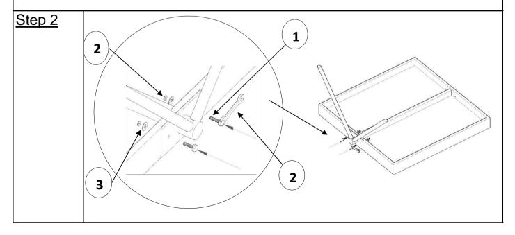
Place the Leg (B) on the Table top (A). Attach the Leg (B) using Long Bolt (1), Spanner (2), Washer (3) and Nut (4). See above picture for reference.
