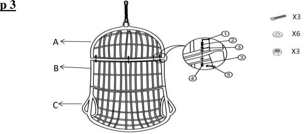
Proceed to assemble Top (A) and Back (B) by using Bolt (②) . Nut (④) and Washer (③) with Allen Key (①) and Wrench (⑤) . Do not tighten.
