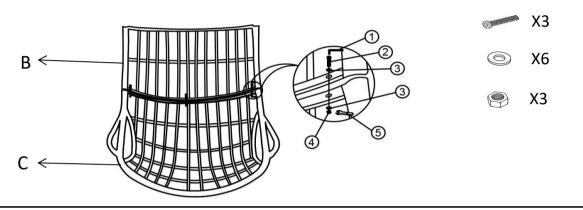
Assemble Back (B) and Seat (C) by using Bolt (2). Nut (4) and Washer (3) with Allen Key (1) and Wrench (5). Do not tighten.
