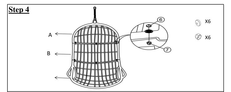
Tighten all screws and nuts . Then add the Nut Caps( 6 , 7 ) on the 6 Bolts as shown in the picture above.
