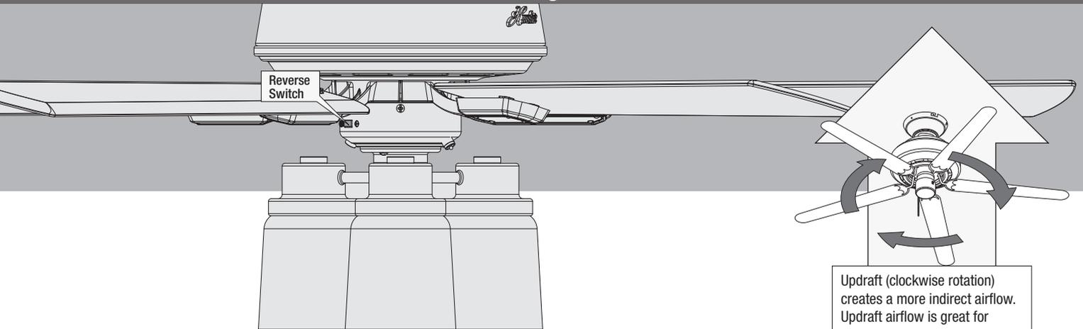
Ceiling fans work in two directions: downdraft (counterclockwise rotation) and updraft (clockwise rotation). To change the direction of air flow, turn the fan off and let it come to a complete stop. Slide the reversing switch to the opposite position. Restart the fan.
