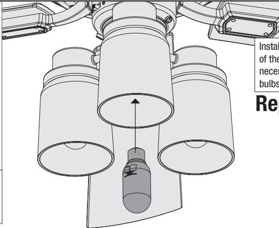
Install a bulb into each of the sockets. When necessary, replace with bulbs of same wattage.
