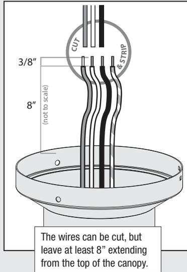
The wires can be cut, but leave at least 8" extending from the top of the canopy.
