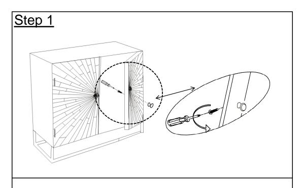
With help of your adult partner, carefully stand the Cabinet. Install the Knob (8) on the Door with the help of Screwdriver (1) as pictured above. Repeat the step to attach the remaining Knob (8) on the Door.
