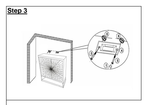
Attach Brackets (4) to Wall Plugs (6) using Wall Plug Screws (5) with Screwdriver (1).
