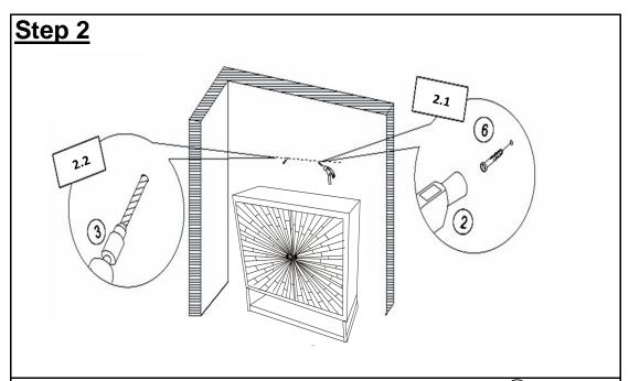
2.1) Drill two holes on wall at same height as Brackets (4) on Cabinet with Power Drill (3).
