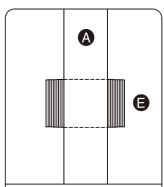
Please ensure threaded cylinders (#E) are popping out on each ends of panel (#A) by approximately 0.4 inches so there is enough threading on each ends of panel (#A) to secure poles.
