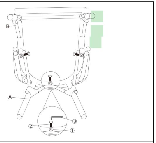
Open the carton and place all the parts onto a clean, non-marring surface. Attach the Seat/Leg(B) to the Backrest/Leg(A) with Washers(1) and Bolts(2) using the Allen Key(3) as shown above.
