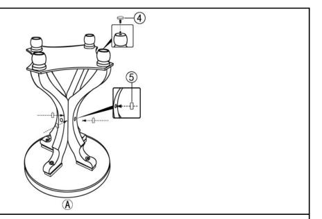
Attach Adjustable Leveller(④) to the Feet (E) by hand. Attach Resin Plug(⑤) to the middle of Leg(C) by hand.
