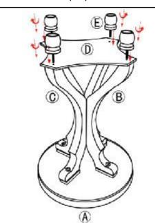
Attach the Shelf(D) to the end of the Protruding Leg(B) and Leg(C), slightly adjust the Protruding Leg(B) and Leg(C) so that the screw mounting positions on the Protruding Leg(B) and Leg(C) are lined with the mounting positions on the Shelf(D).
