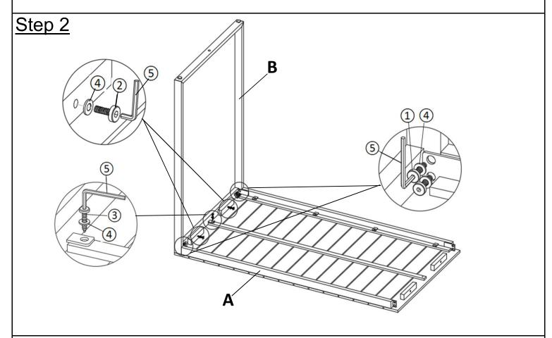
Attach the Leg Frame (B) to the Table Top (A) using Bolts (1,2) and Screws (3) with Washers(4) and the Allen Key(5) as shown in the picture above. Repeat the same process with the remaining Leg Frame (B).
