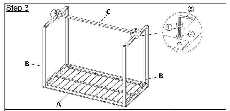
Attach the Leg Connector (C) to the Leg Frame (B) using Bolts (1) and Washers (4) with the Allen Key (5) as shown in the above picture.
