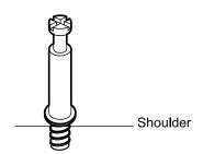
Tighten Until Shoulder is flush with panel.Do not overtighten or undertighten (see example below).
