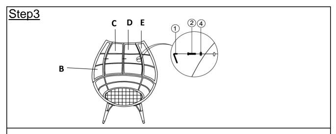
Attach the Left Panel (B), (C) to the Right Panel (D), (E) using Bolts (②) and Washers (④) with the Allen Key (①) as shown in the picture above.
