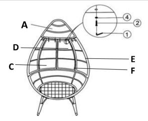
Attach the Top Panel (F) to the Left Panel (C), (D) and the Right Panel (E), (F) using Bolts (2) and Washers (4) with the Allen Key (1) as shown in picture above.
