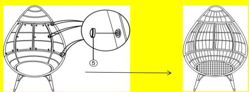
Add the Nut Caps ( (5)) onto the Bolts as shown in the picture above.
