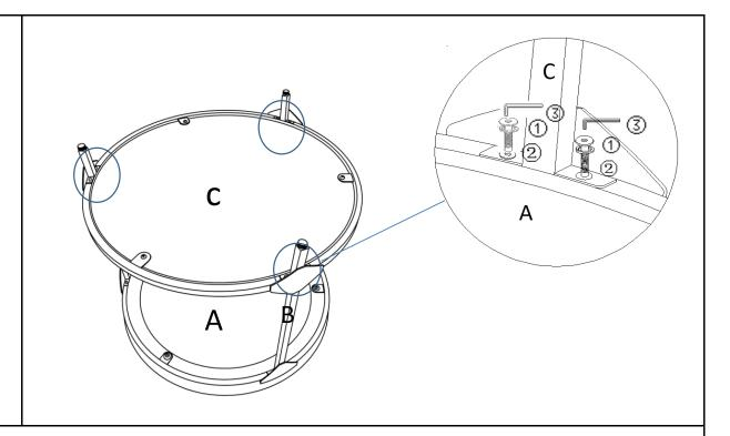
Attach the Leg(B) to the Base Plate(C) using Bolts(1) and Spring Washers(2) with the Allen Key(3).
