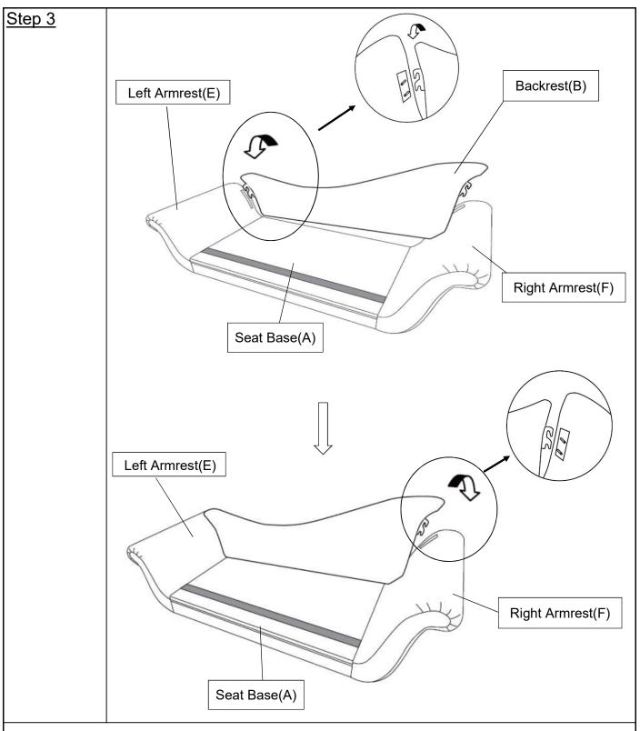
Standing behind the Seat Base(A) while holding Backrest(B). Hang on the hook of Backrest(B) onto the Preserved bolt of Left Armrest(E) as shown above, make sure two hooks are both on top of Preserved bolt.
