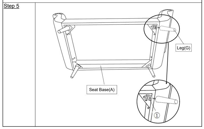
Install the Leg(G) into the bottom of Seat Base(A) by placing Plastic Washer(1) on the threaded stem. Then insert threaded stem into the threaded mounting postion at the bottom of Seat Base(A). Tighten by turning the Leg clockwise.
