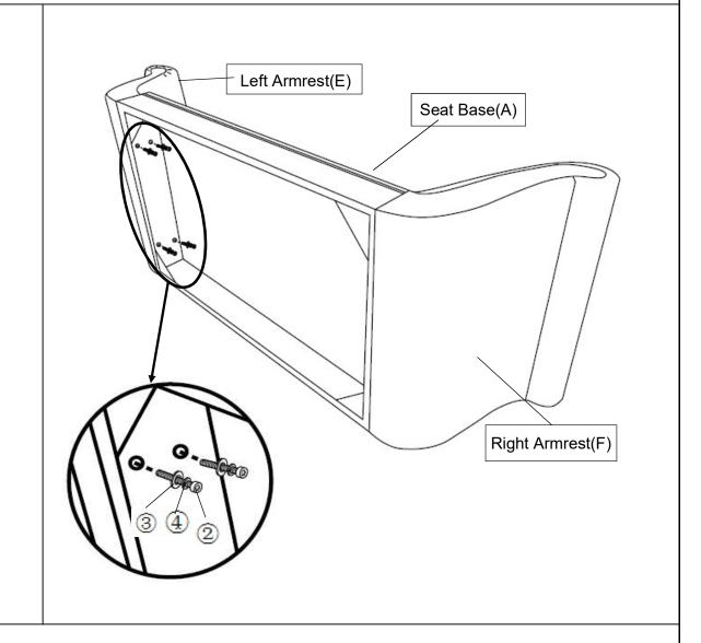
Attach the Left Armrest(E) to Seat Base(A) using Bolt(②),Spring Washer(④),Flat Washer(③) and turning clockwise by hand .
